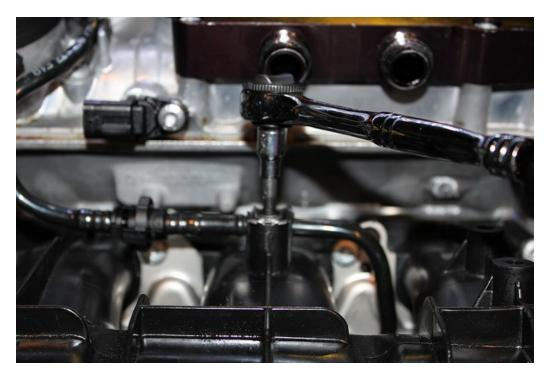
10) Remove Lower Bolt from Manifold Brace & Remove Brace (not to be re-used, silver bolt left of throttle body):
