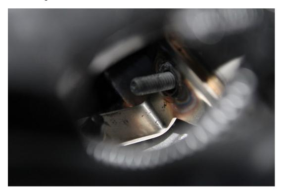
18) Remove Silver Bolts Holding Manifold to Cylinder Head:
