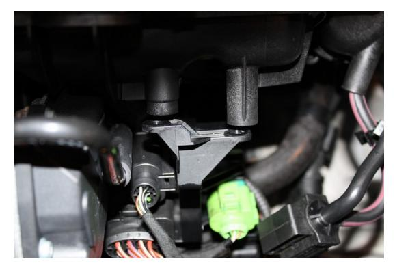
16) Remove Nut Holding Fuel Rail Behind Bracket:
