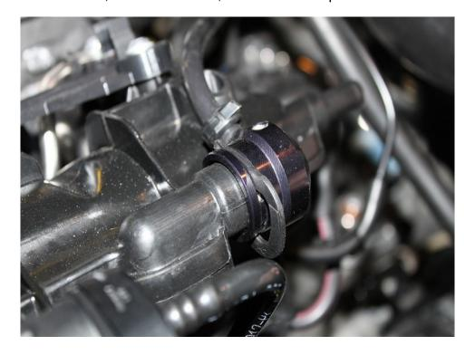
5) Remove Connectors On Valve Cover:
