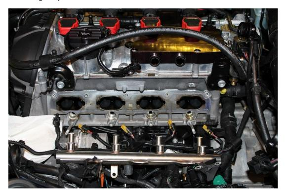
NOTE: Carbon Buildup (5,000 miles on new engine):
