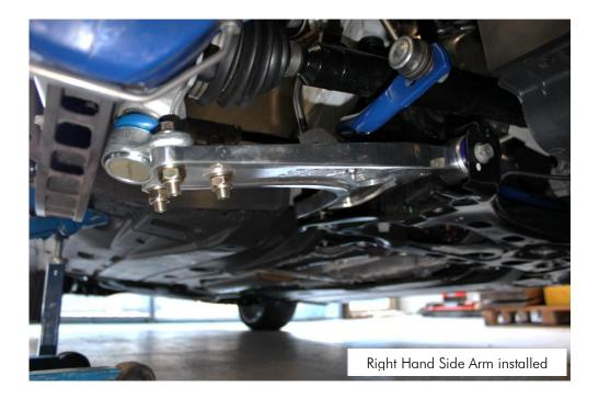
• Tighten all bolts to manufactures torque setting and carry out wheel alignment.
