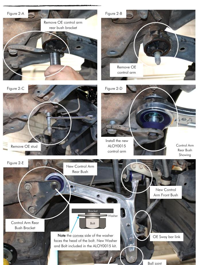
Figure 2 – View from underneath of the vehicle of the Left Hand Side New Control Arm ALOY0015 installation
