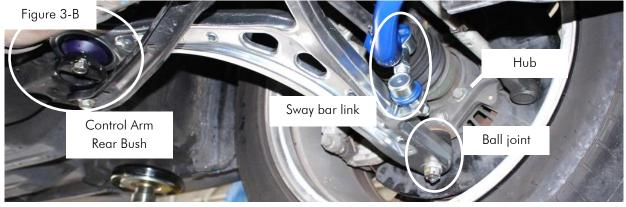
Figure 3 – View from underneath of the vehicle - Left Hand Side Control Arm installed
