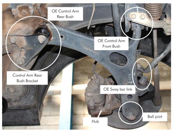
Figure 1 – View from underneath of the vehicle of the Left Hand Side OE Control Arm
