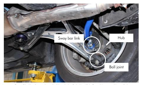
$Figure\ 01-View\ from\ underneath\ of\ the\ vehicle\ -\ Right\ Hand\ Side\ Control\ Arm\ assembly\ installed$
