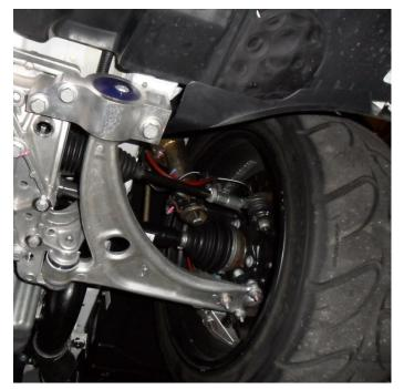
Figure 03 - View of underside of car right hand side shown with arm assembly installed
