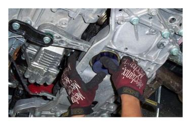
2. Use the grease supplied to cover the new polyurethane bush and insert the bush into the mount, making sure the voids line up. Once the bush is started a soft face hammer can be used to tap the bush all the way in.
