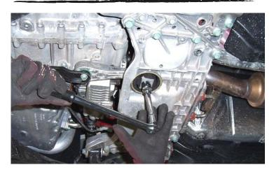
1. Using a 21mm socket/spanner remove the rear engine support centre bolt that is mounted in the aluminium sub frame.
