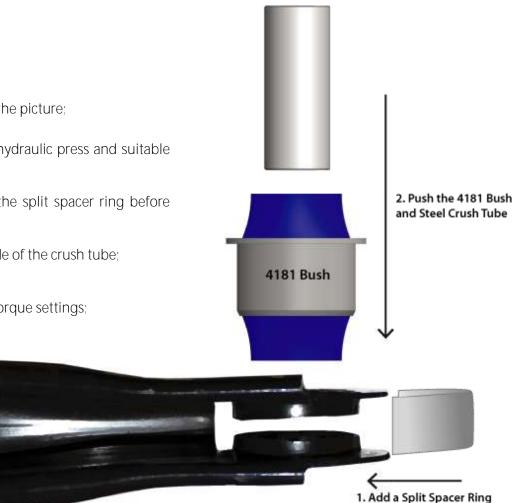
*Note:* Polyurethane bushings must be fitted to both sides of the vehicle. This kit should be installed by a Qualified Motor Mechanic.
