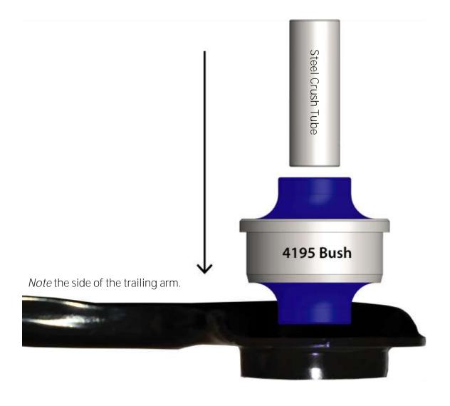
*Note:* Polyurethane bushings must be fitted to both sides of the vehicle. This kit should be installed by a Qualified Motor Mechanic.
