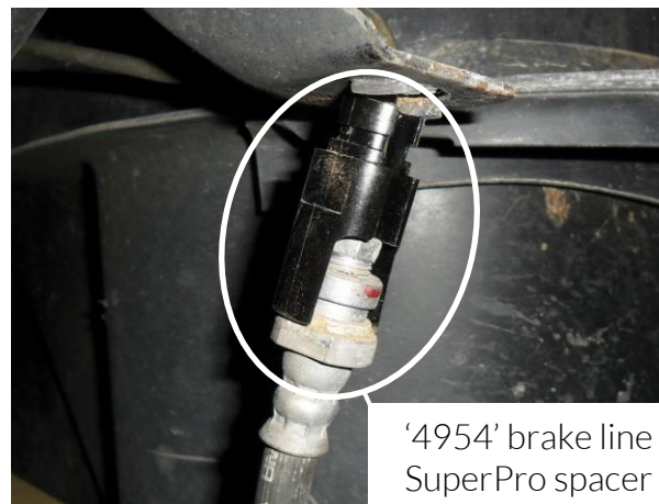
Figure 03 – Installing '4954' brake line spacer
